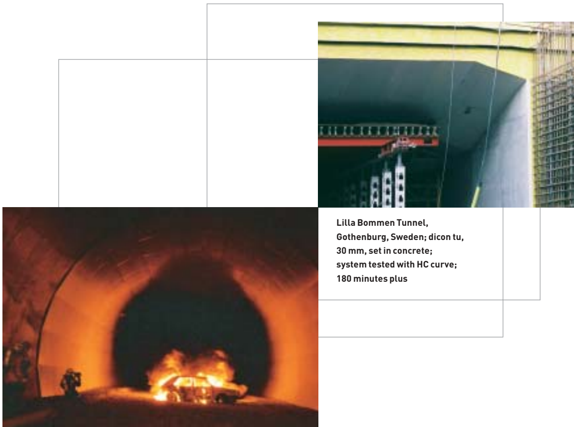
Tunnel des Bruyères, fire drill; structural concrete protected with AESTUVER dicon tu fire-resistant boards in test area
