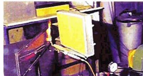
Radiant panel for testing reaction to fire
