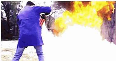
Test of the efficacy of a portable extinguisher on a hearth of type B (liquids)
